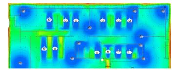
**Figure 3.** Utilizing the M2M communications, a Rajant solution only needs to utilize 10 infrastructure and a few mobile machine nodes to provide complete coverage to the entire indoor industrial space. Why? Because Rajant BreadCrumbs transmit at much higher Tx power than typical Wi-Fi, providing significantly better coverage while M2M allows robots, and anything mobile, to extend coverage and fill coverage gaps.
