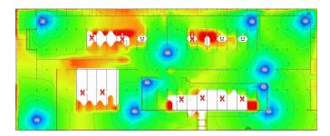
**Figure 1.** An enterprise Wi-Fi solution using 10 infrastructure pieces is unable to cover the entire indoor industrial space. Clients on mobile machines are unable to connect and entire corridors are left without coverage.
