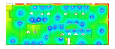
**Figure 2.** The solution to provide coverage for the entire floor of an indoor facility using a traditional enterprise Wi-Fi technology is to add in more nodes. The total number of infrastructure is now at 35 nodes to completely cover the area.
